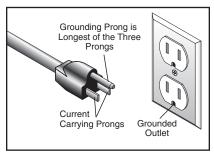
**Figure 1.** Typical type 5-15 plug and receptacle.
